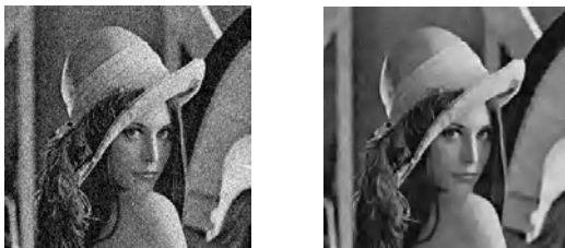
Fig. 3. NL-means denoising experiment with a natural image. Left: Noisy image with standard deviation 20. Right: Restored image.
